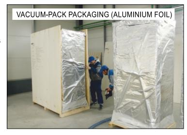
We are using all types of packing foils, shock, temperature, bending and moisture sensors, VCI COR-PACK tablets, desiccant bags and textile anchorage straps.
